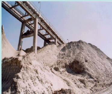
Stockpiles of waste gypsum
